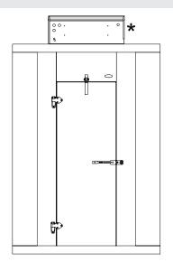
These systems include ambient controls, weather-proof hoods, precharged systems with quick connects for simple field connections to precharged lines of your choice. Consult factory for application, pricing and ship date availability.
