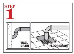
Connect the drain pipe from scrap accumulator to floor or wall drain.
