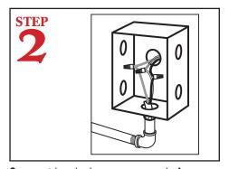
Connect hard wire power supply from dishmachine to power box.
