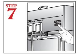
Press and hold the Fill/Start Switch until the water level is approximately 1/2" to 3/4" below the overflow hole in the PVC standpipe.
