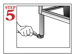
Level dishmachine by adjusting leveling legs. Dishmachine must be level front and back.
