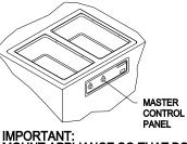
MOUNT APPLIANCE SO THAT BOTH THE CONTROL PANEL AND DRAIN MANIFOLD ARE LOCATED TO THE FRONT OF THE FIXTURE.
