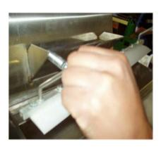
Tighten the screws on the safety shield.
