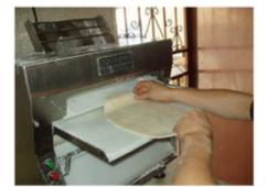
Pass 2 Is just like the first pass, but this time, turn the dough 90 degrees left or right, inserting it into the bottom rollers. After the doughball is rolled out, place hands or receiving tray beneath the bottom chute. Lightly stretch dough to the desired size after placing it directly onto a pan, screen, or peel.
